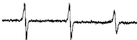
Fig. 5. ESR-spectrum of the nitroxide radicals formed in the cross-coupling reaction between III and TNM + diethyl acetamidomalonate.
